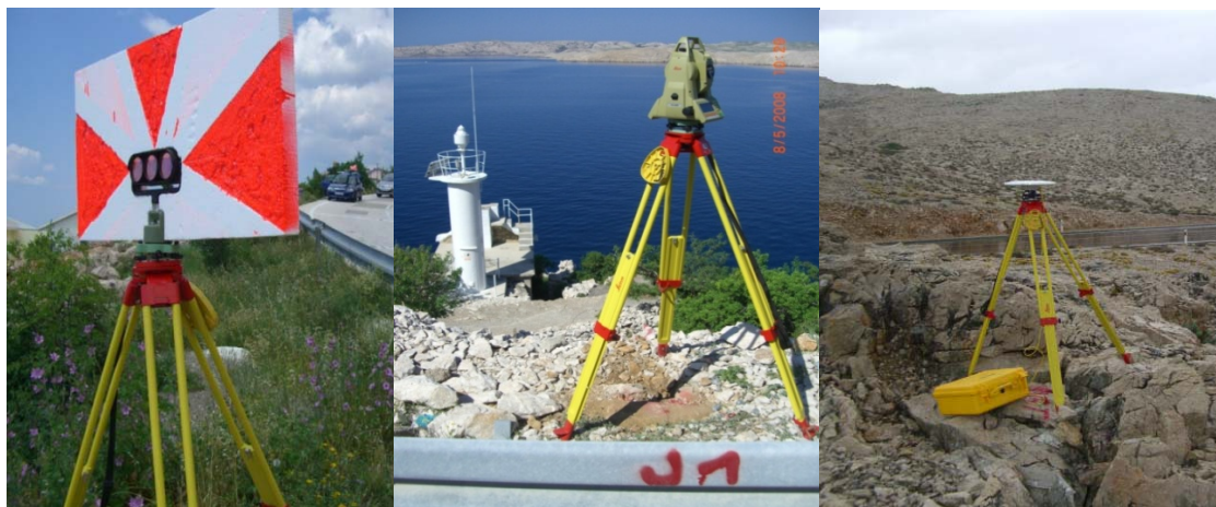
Figure 2: Devices for trigonometric and GPS levelling
